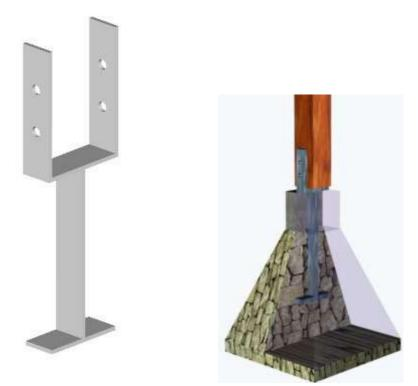
It is essential that a wood frame structure mounted on a concrete frame/brick stub wall must be fully anchored together. A bracket, as shown above left, made of non-corrodible metal, must be cast into the bearing structure to provide a structural connection for the whole wall through to the foundation. The wood column must be bolted to the bracket as shown, and the bracket must be fully secured into the concrete as shown on the right.
