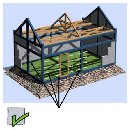
**Good tying practice.** An illustration for a reinforced concrete frame building, where metal ties are used to tie walls to the main building structure. Steel wall ties are to be at maximum of 40cm spacing and a minimum of 8mm diameter, and bent at the end. They are for all openings in the walls.
