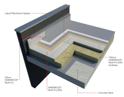
HARDROCK<sup>®</sup> Multi-Fix (DD) is supplied with an integral glass mineral fibre facing which provides a compatible surface for the application of polymeric and elastomeric liquid membrane systems.
