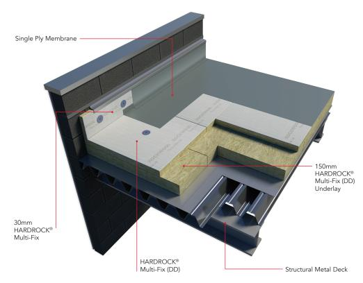
HARDROCK<sup>®</sup> Multi-Fix (DD) roofing boards are perfect for mechanically fastened single-ply and EPDM systems.
