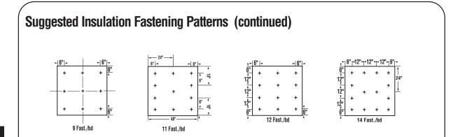
Fastener Placement for 4' X 8' Boards
