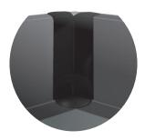
**6.** Cut a piece of RubberShell in accordance to the illustraion and weld it into the middle of the corner, also overlapping the top corner.
