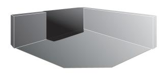
2. Apply the second flashing strip; heat-weld the overlap and onto the roof side.
