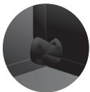
**4.** Remove the remaining release film. Fold the unwelded flaps together in a V-shape and heatweld.
