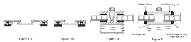
Figure 11. Depiction of Typical Two-Part Metal System Connecting Profiles Currently Used
