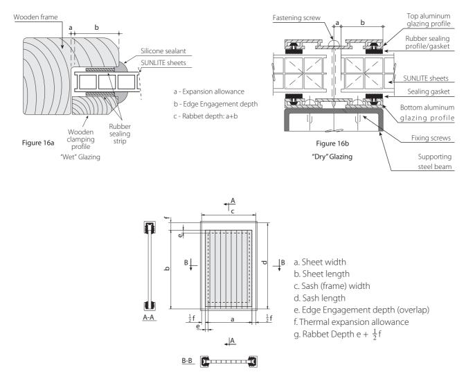
Figure 16c. Schematic Sketch of Rebbet depth and Expansion Allowance. ("wet" and "dry" methods)
