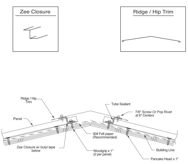
Panels should end parallel to the ridge. Attach zee closure parallel to closure ridge. Fasten hip/ridge trim to the zee using #14 x 7/8" Lap/screw. Caulk, lap (minimum of 6" hooking the hem) and fasten the subsequent trims.
