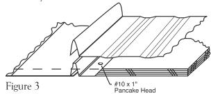
5. Lightly compress and snap panels together at seam. Snap panels from eave to ridge. Screw the second panel in place using 1" pancake head screw in the male edge fastening flange.
