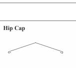
Place a short section of ridge cap on one end of the peak so it lies evenly side to side. Mark the outside edges, then repeat the process at the other end. Snap chalklines between the marks, and set the ridge cap on these lines as it's installed. Exposed Valley Trim (details page 16.1)
