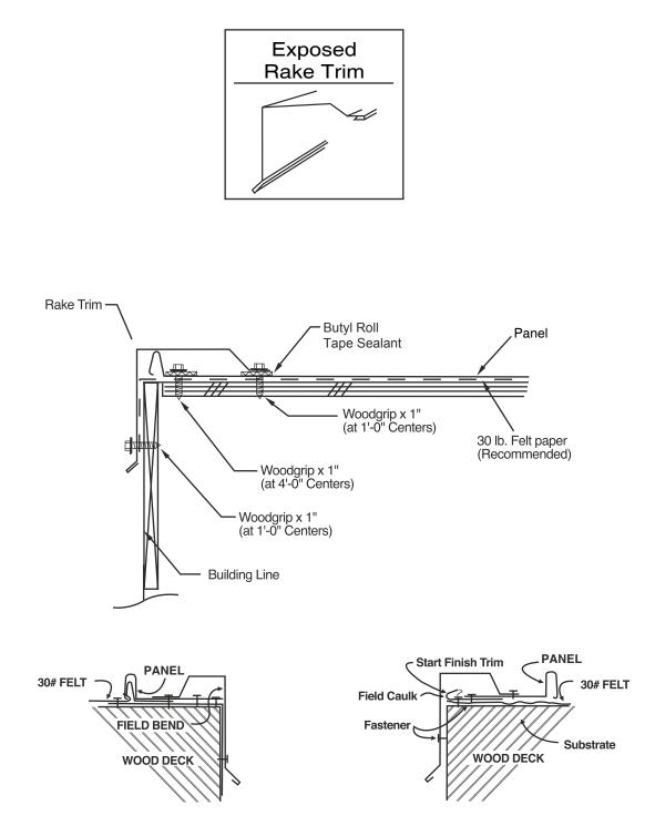
Begin by aligning Standing Seam panel flush to the gable end of the building and attaching the flange side of the panel with pancake head screws. Assemble the Exposed Rake Trim with #10 x 1" washered screws as shown with screws 18" to 24" apart.
