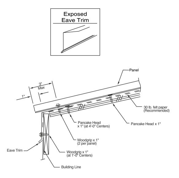
Attach eave trim as shown with  $#10 \ge 1$ " low profile pancake fastener. Open the hem of the next trim for approximately 4". Caulk and lap the trim a minimum of 3" hooking the hem. Install panel and fasten at eave with  $#10 \ge 1$ " Woodgrip screw. Additional ice and water shields may be required if climate is extreme.
