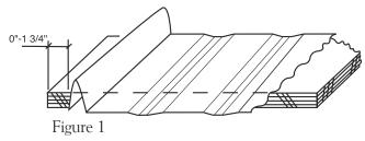
2. Panels should be installed perpendicular to ridge for ridge trim attachment.
