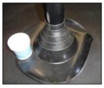
Cut the PS Pipe Seal above the raised "rib" one size smaller than the pipe diameter. DO NOT CUT DIAGONALLY THROUGH THE RIB. Pull pipe seal over pipe until base flange is in contact with the EPDM membrane.
