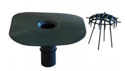
These are 68mm roof outlets designed to be inserted into the existing 68mm diameter down pipe. The outlet is fitted with an anti-backup seal to achieve a watertight join. The outlet is attached to the membrane using 225mm PS uncured flashing tape. A Leaf grate for this outlet is also available.
