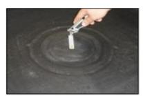
2) Find the locating pin on the protective cap, place cutting guide over the pin and cut round the circular plate.
